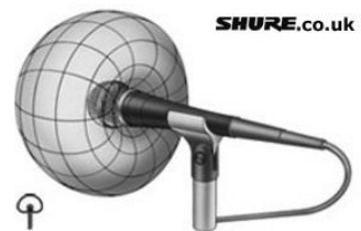
Microphone Pickup Pattern
