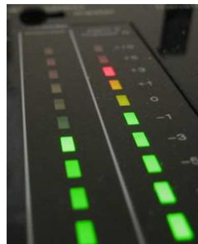
The signal displayed on the right side is starting to clip (shown in red)
